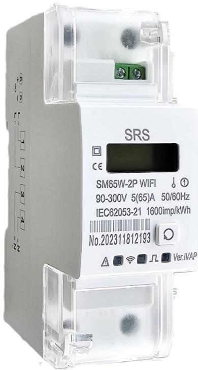
The meter is used in three phase four wire power grid. It is designed to measure AC active energy and variable parameters. It has remote read communication to port RS485 and WIFI, and a long-life with the advantage of high stability, high over load capability, low power loss and small volume.
